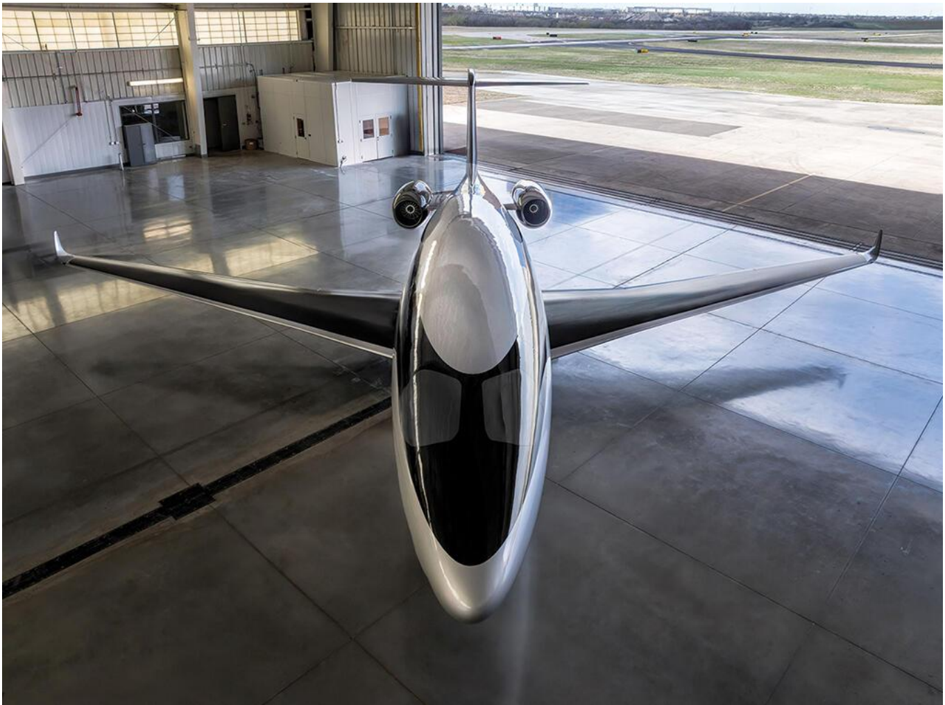
A smooth, step-free surface finish is essential to sustaining drag-reducing laminar flow. Credit: Otto Aerospace
